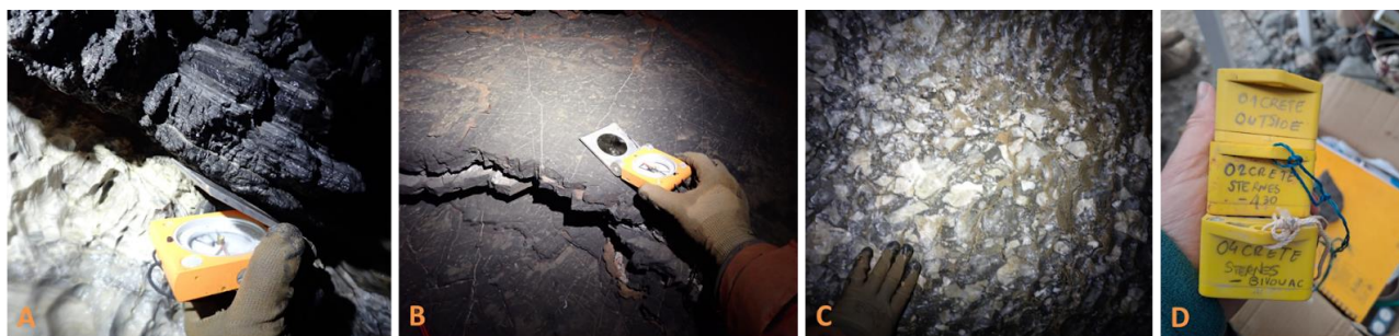
Measurements of the inclination and orientation of different rocky types with the use of a geological compass (A,B), a type of pyroclastic rock (C) and the three detectors placed inside the cave (D).
